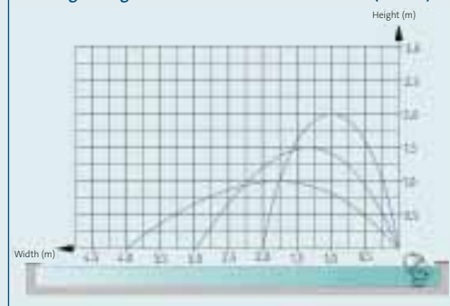
Jet length diagram with OASE recommendation (indoor)
