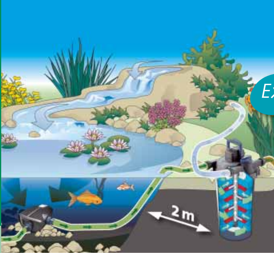
Schematic diagram: Pressure filter FiltoClear in combination with filter and watercourse pump
