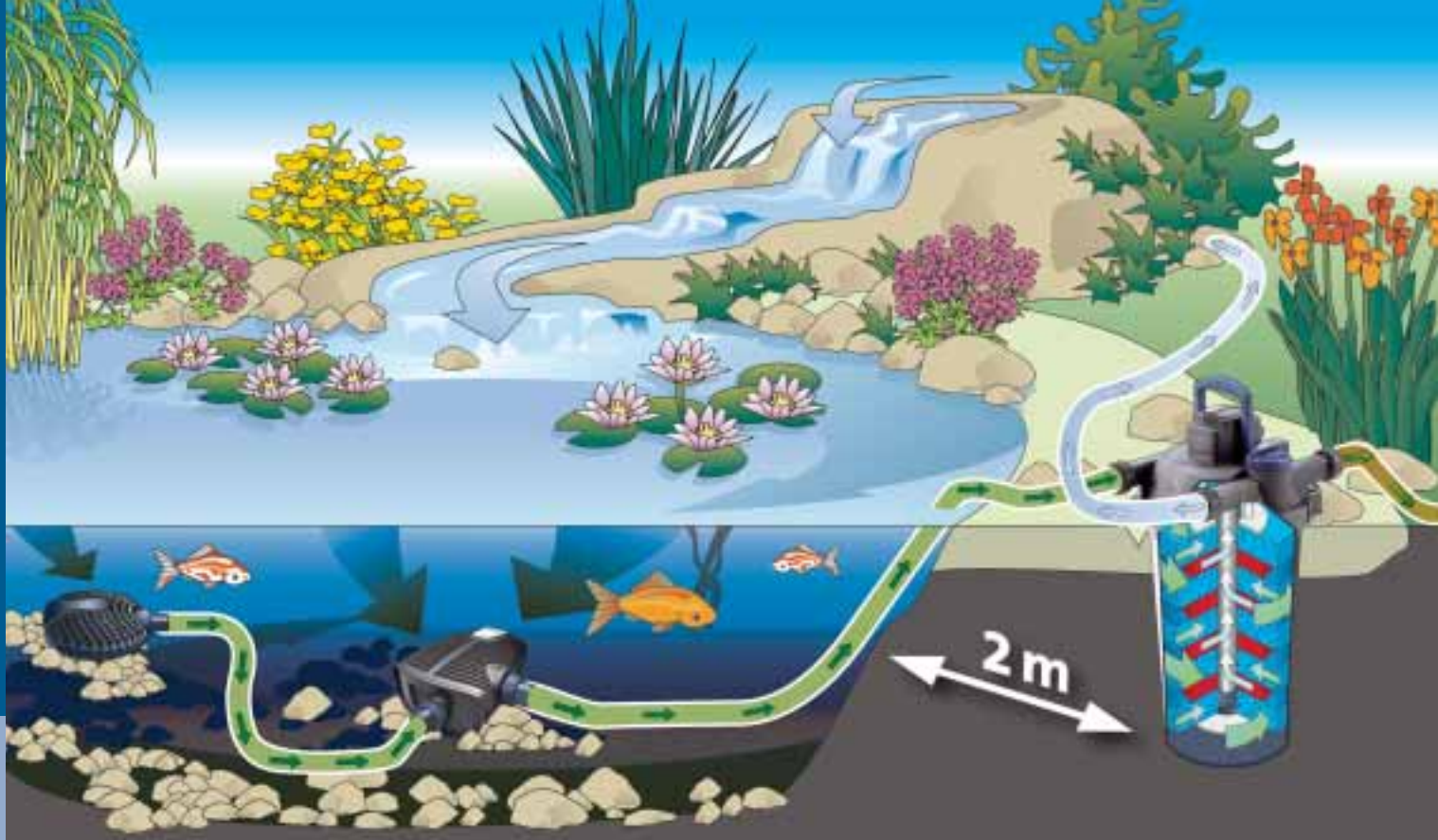
Schematic diagram: Filter and watercourse pump AquaMax Eco (PRO) in combination with an OASE pressure filter FiltroClear (PRO)
