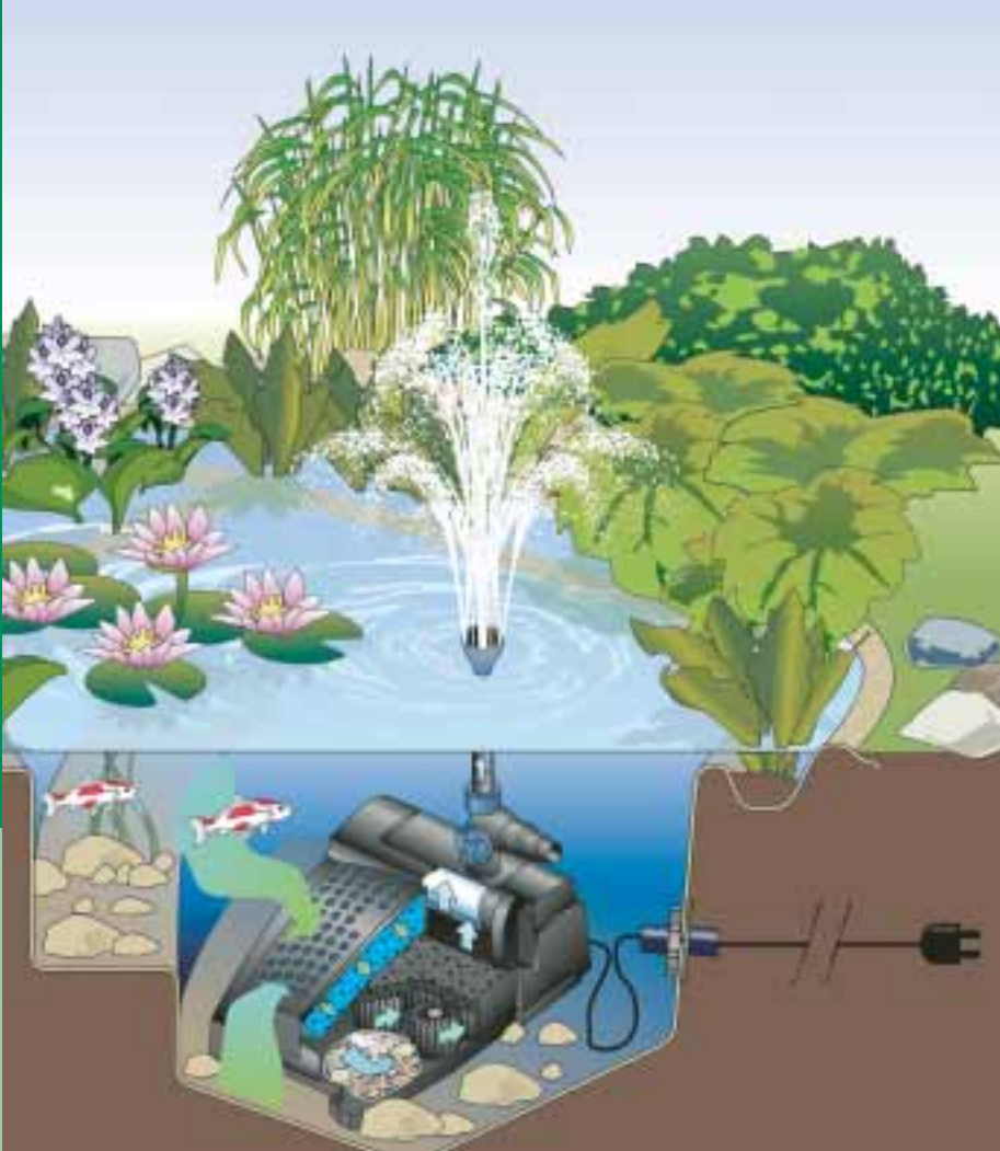
Schematic diagram: Underwater filter Filtral UVC inserted in a pond
