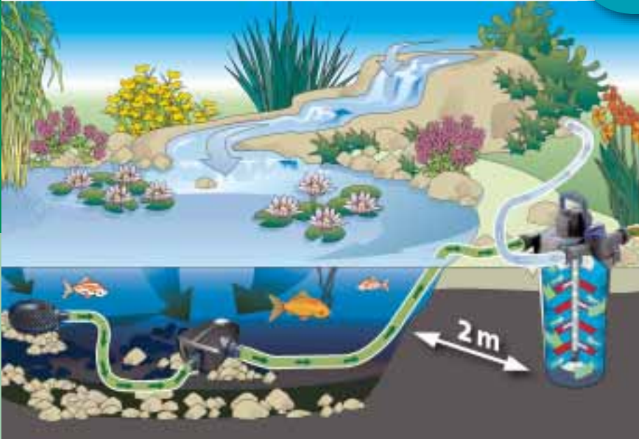
Schematic diagram: Pressure filter FiltoClear in combination with filter and watercourse pump
