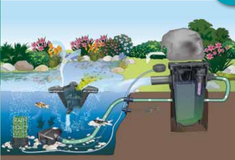
Schematic diagram: Interaction of the different CWS components
