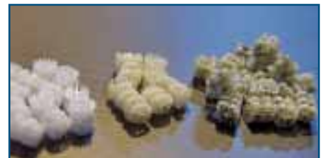
Biological surface for settlement of the microorganisms (left – biomedes that has not yet been used, right – with settled microorganisms).
