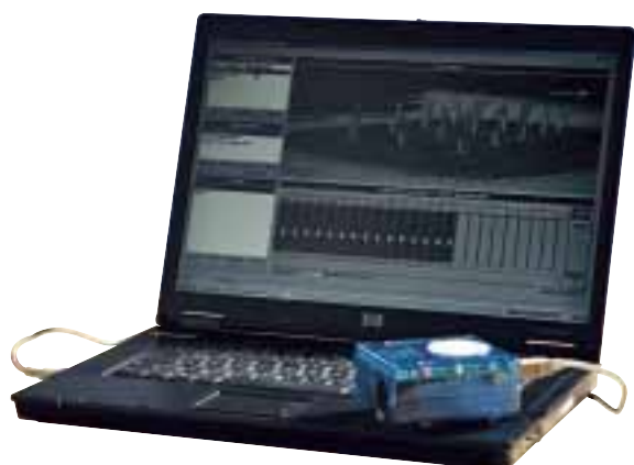
The OASE Easy Control can program your system from a PC or laptop.
